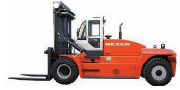
FDE200/230/250-12 -Capacity: 20t-25t -Engine: Cummins -Transmission: ZF
