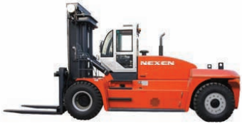
FDE135-9 -Capacity: 13.5t -Engine: Cummins -Transmission: ZF
