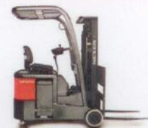
FBAT10/12 -Capacity: 1.0t/1.2t -Controller: AC -Transmission: ZF -Motor: Schabmuller
