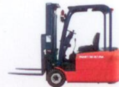
FBAT 16/18/20 -Capacity: 1.6t/1.8t/2.0t -Controller: Zapi -Transmission: ZF -Motor: Schabmuller
