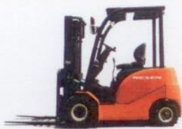
FBA15/18 -Capacity: 1.5t/1.8t -Controller: Zapi -Transmission/ Motor: KDS -Drive: Single/Twin
