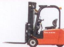
FBAT16RD -Capacity: 1.6t -Controller: Zapi -Transmission: ZF -Motor: Schabmuller
