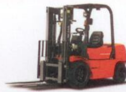
FDR30/35 -Capacity: 3.0t/3.5t -Engine: Yanmar 4TNE92/94/98, Mitsubishi S4S, Cummins QSF2.8L -Transmission: STD/OKA/MSP
