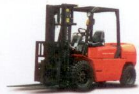
FDR40/45/50s -Capacity: 4.0t/4.5t/5.0t -Engine: Nissan TD42, Perkins 1104D -Transmission: STD
