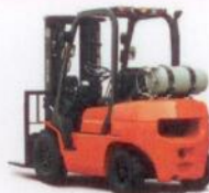
FGR30/35 -Capacity: 3.0t/3.5t -Engine: Nissan K21, Impco Nissan K25, Impco -Transmission: NNT/OKA/MSP
