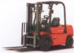
FDR20/25 -Capacity: 2.0t/2.5t -Engine: Yanmar 4TNE92/94/98, Mitsubishi S4S, C240 Cummins QSF2.8L -Transmission: STD/OKA/MSP
