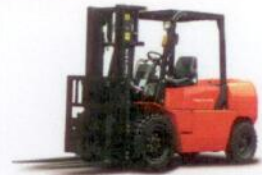
FGR40/45/50s/55 -Capacity: 4.0t/4.5t/5.0t/5.5t -Engine: GM 4.3L, Impco -Transmission: OKA
