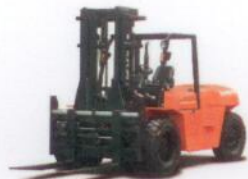
FDR80/100 -Capacity: 8.0t/10.0t -Engine: Cummins QSB4.5 T111A Isuzu 6BG1 -Transmission: STD
